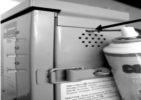
Figure 3. Cover is closed and CO nozzle is inserted, all the way in, through one of the TOP holes found on the RIGHT SIDE of the case. Do not insert nozzle through FRONT vents because the CO gas will be rapidly deflected back.
